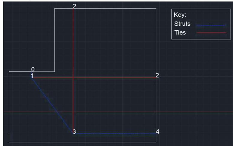
Figure 2: STM layout and node numbering for STM E.9.
