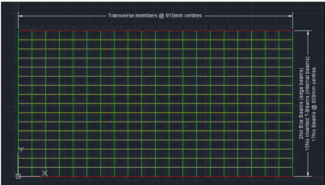
AutoCAD sketch of the above grillage showing spacing of grillage members.
